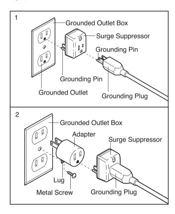
The temporary adapter should be used only until a properly grounded outlet (see drawing 1) can be installed by a qualified electrician.
